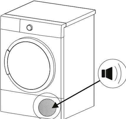
A line drawing of a front-loading washing machine. A circular area at the bottom front is circled, with an arrow pointing to a speaker icon. The speaker icon is a black trapezoid with three curved lines to its right, indicating sound. | <p><b>Sonido del compresor</b></p> <p>Es normal escuchar un sonido metálico del compresor de vez en cuando mientras la máquina está en funcionamiento.</p>                                                                        |
